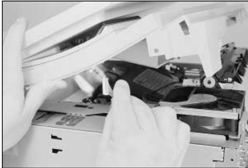
Figure 6-4 Control Panel Cable
