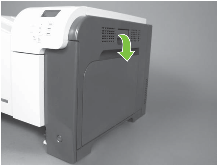
Figure 6-18 Remove the fuser (1 of 2)
