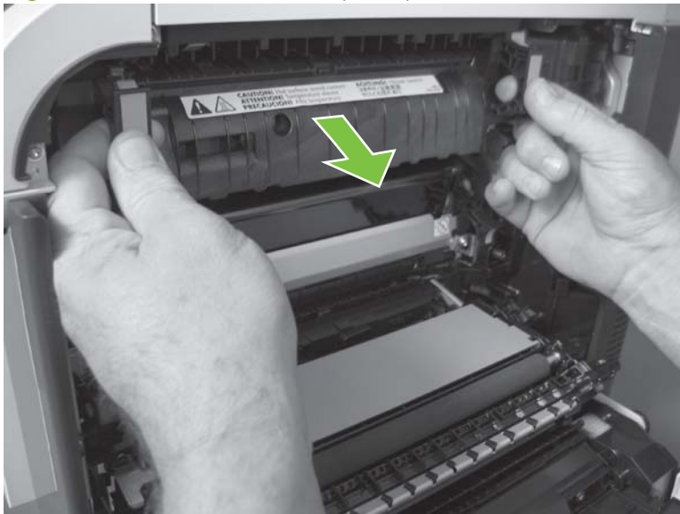
Figure 6-19 Remove the fuser (2 of 2)
